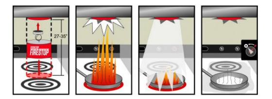
The Stovetop Firestop products are designed for cooktops with a traditional vent-hood and for residences with over-the-stove microwaves. They deliver a fire suppressing powder to both front and back burners. Each product has a six-year effective life.
